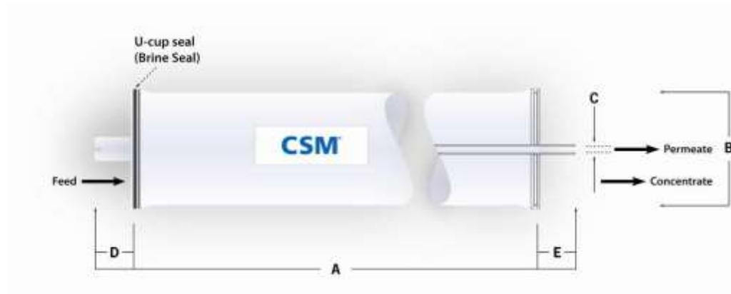
1. Each membrane element supplied with one brine seal, one interconnector (coupler) and four o-rings.
